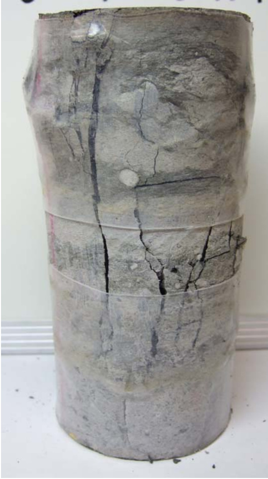
Figure C-12 UCS Specimen DGR4 727.95 m
