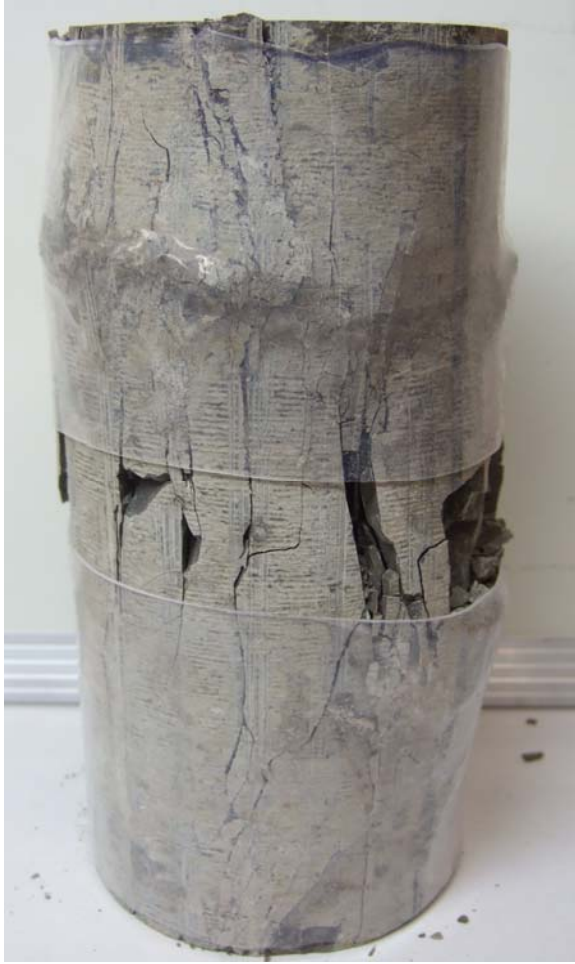
Figure C-14 UCS Specimen DGR4 771.71 m
