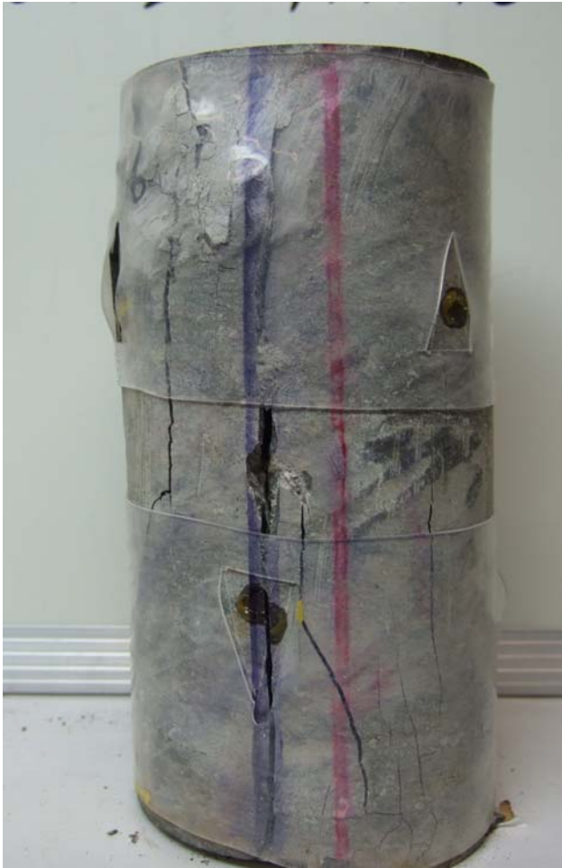
Figure C-4 UCS Specimen DGR5 711.96 m
