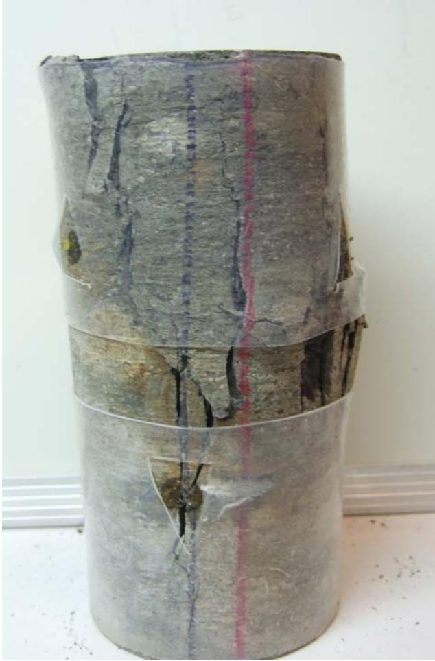
Figure C-3 UCS Specimen DGR4 682.22 m
