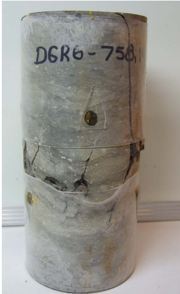
Figure C-9 UCS Specimen DGR6 755.19 m
