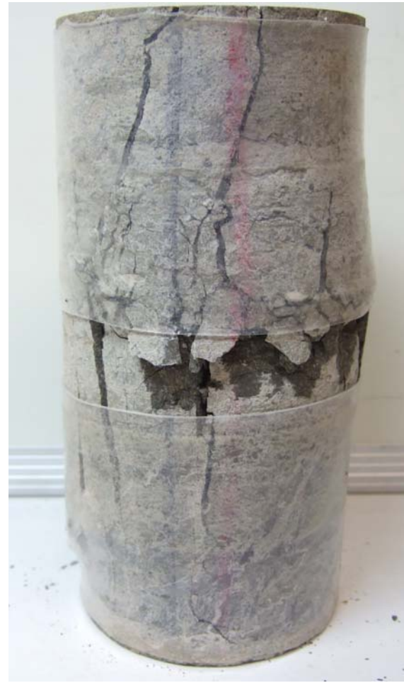
Figure C-17 UCS Specimen DGR4 809.88 m
