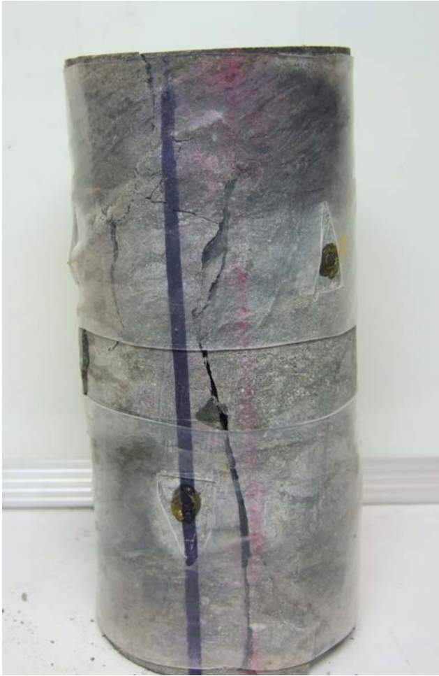
Figure C-6 UCS Specimen DGR5 731.27 m
