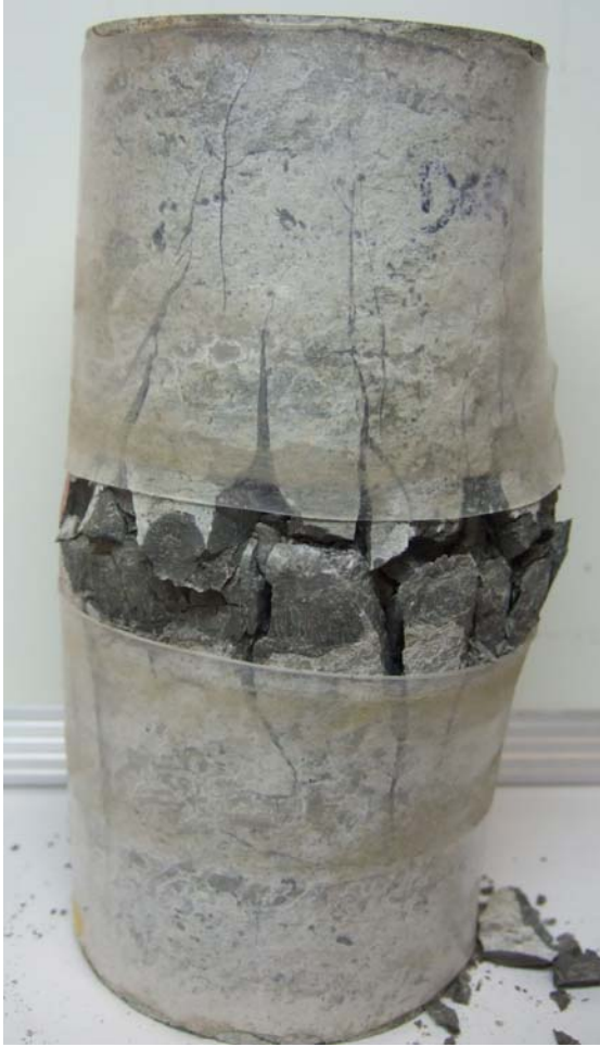
Figure C-16 UCS Specimen DGR4 808.56 m
