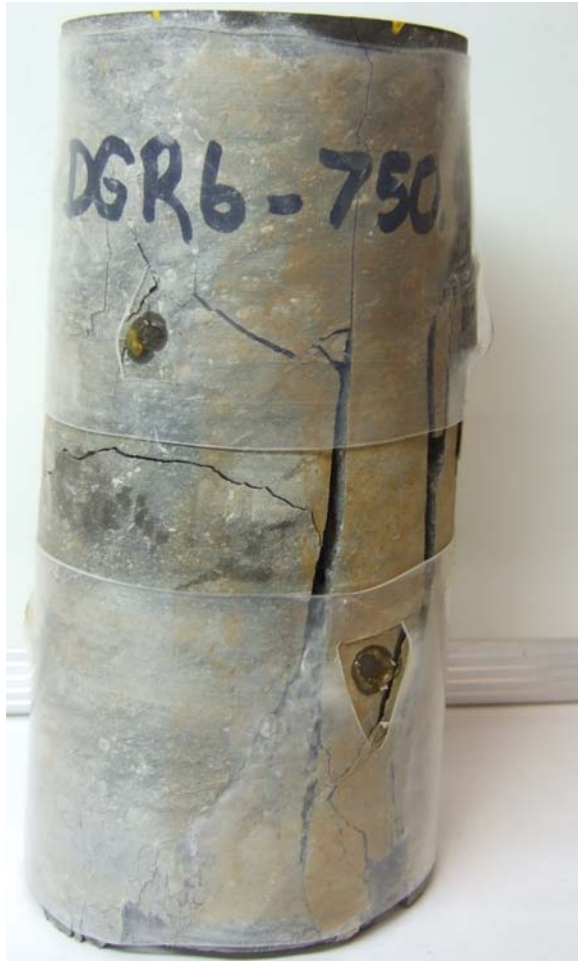
Figure C-8 UCS Specimen DGR6 747.99 m
