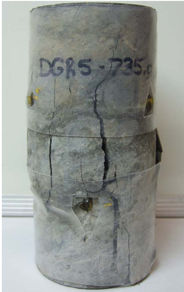
Figure C-7 UCS Specimen DGR5 735.61 m
