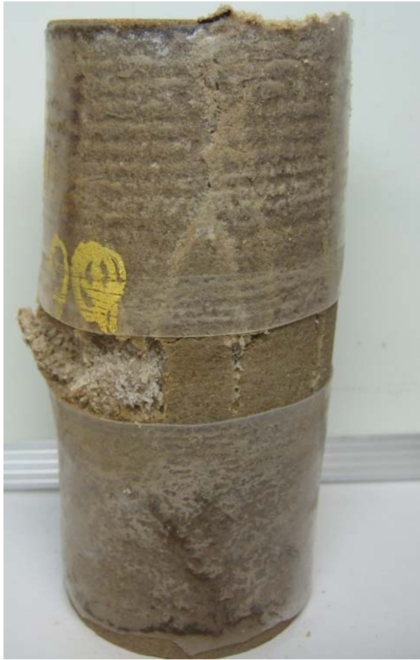
Figure C-18 UCS Specimen DGR4 856.29 m
