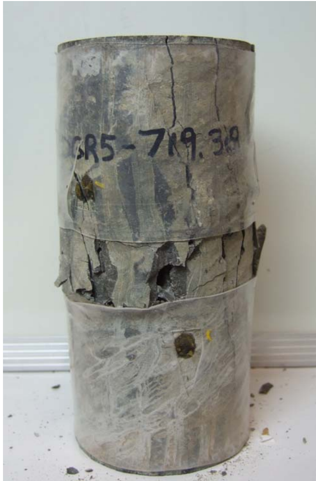
Figure C-5 UCS Specimen DGR5 719.38 m
