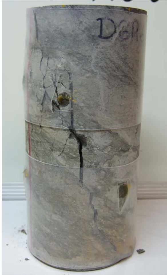
Figure C-11 UCS Specimen DGR6 773.82 m
