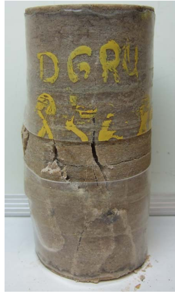
Figure C-19 UCS Specimen DGR4 856.80 m
