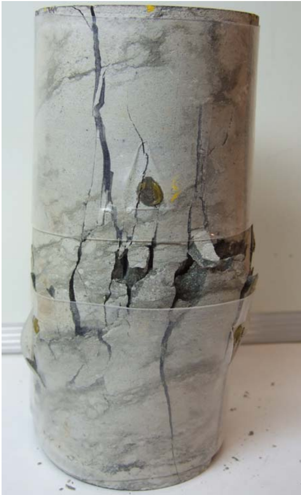
Figure C-10 UCS Specimen DGR6 770.07 m
